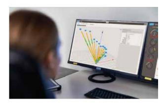
For longhole drilling, OptiMine® Drill Plan Visualizer shows existing plans and actual drilling results in a 3D format, including measurement while drilling (MWD) data, when available.
